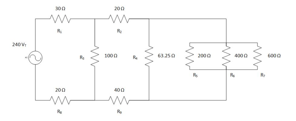
Find  $V_T$ ,  $R_T$  and  $I_T$  as well as Voltage, Resistance and Current Values for each resistor.
